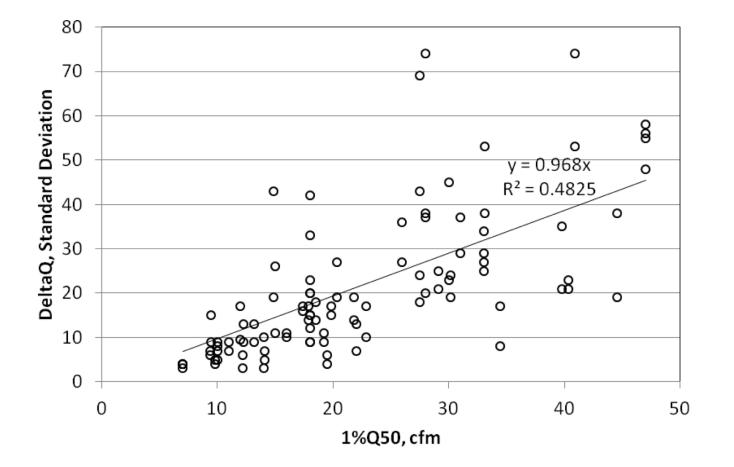
Mean difference between rule of thumb and measured results is 1 cfm RMS difference is 11 cfm
