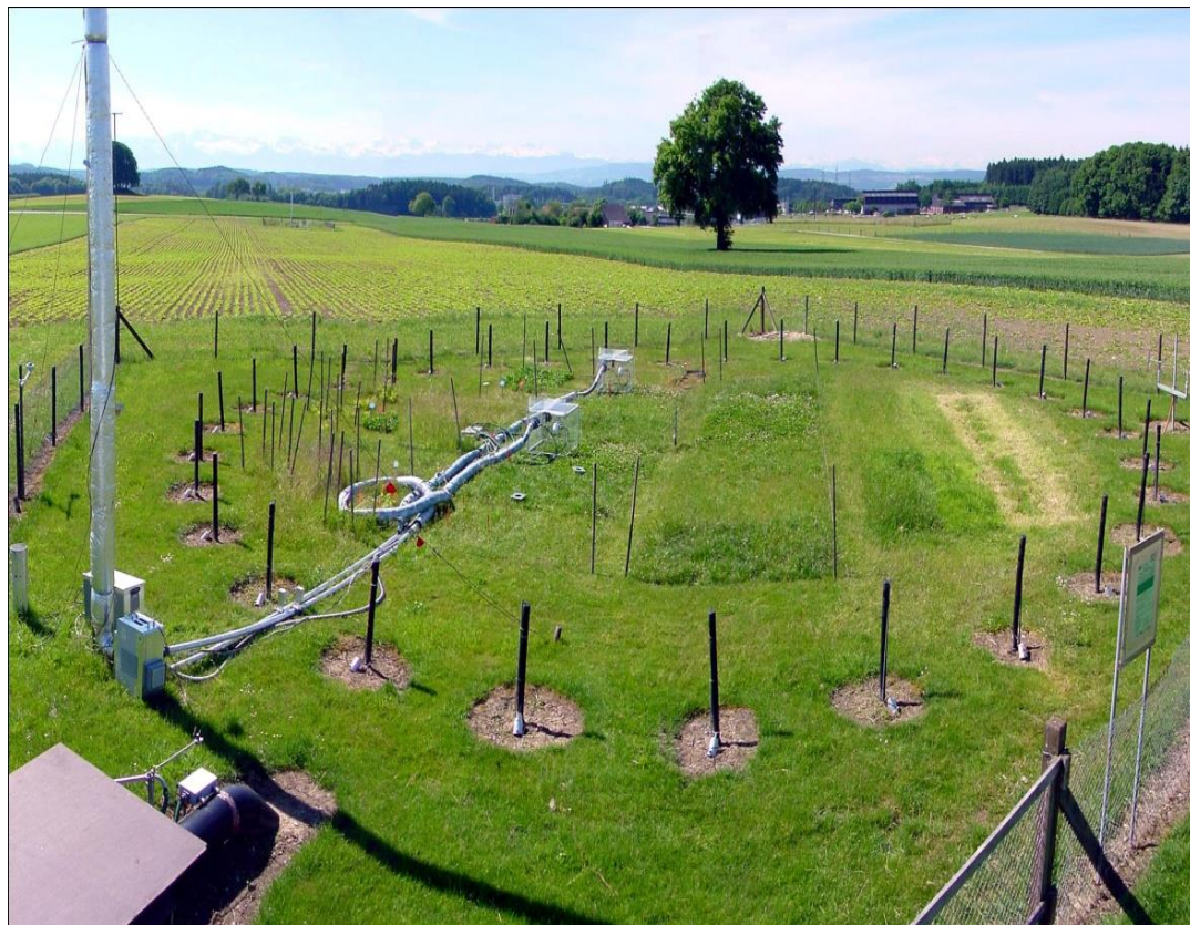
FACE experiment to assess the impact of elevated [CO 2 ] on soil C sequestration
