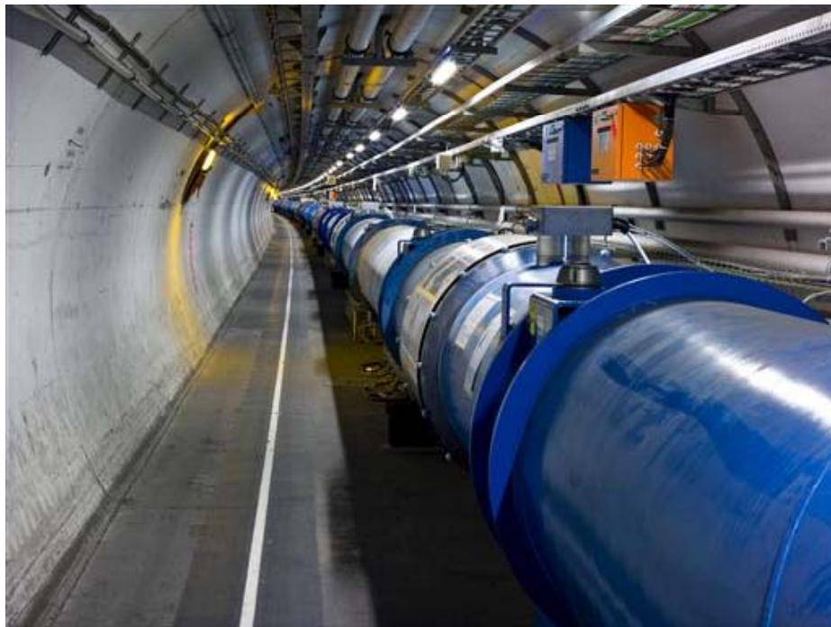
The LHC Tunnel, showing superconducting bending magnets
