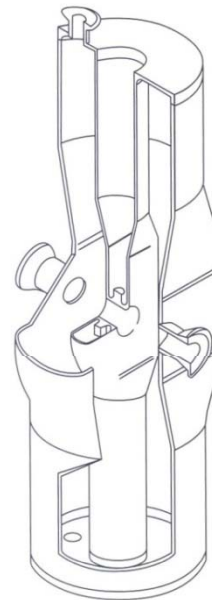
Figure 4.26 350-MHz \beta = 0.12 coaxial half-wave resonator with a single loading element (courtesy of J. R. Delaven, Ref. 33).
