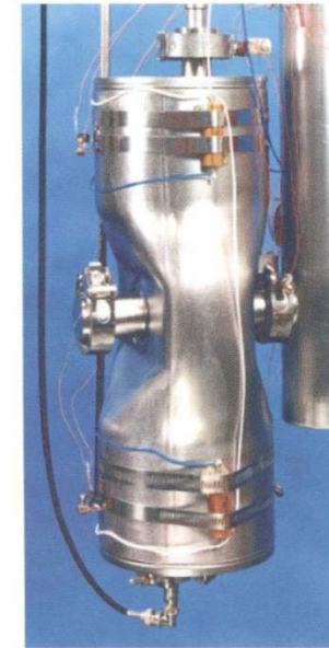
Figure 4.26 350-MHz \beta = 0.12 coaxial half-wave resonator with a single loading element (courtesy of J. R. Delaven, Ref. 33).
