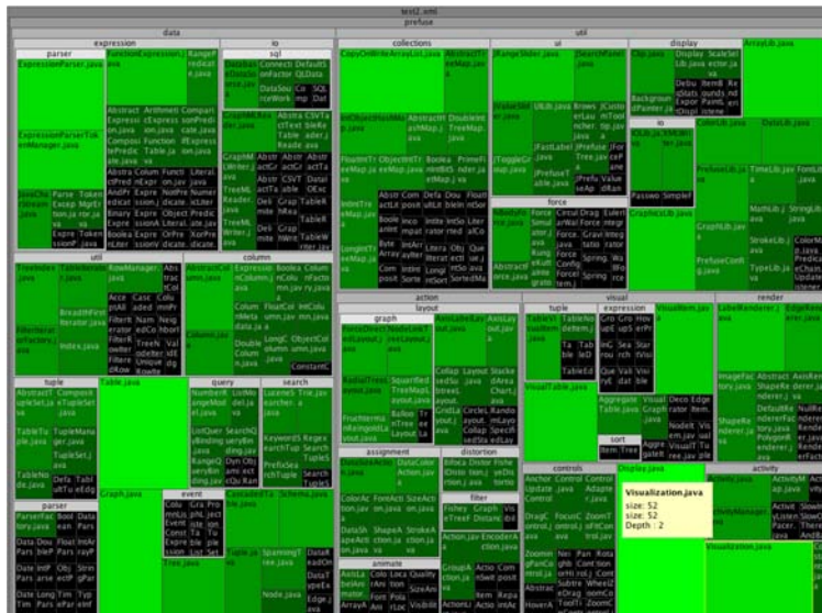
Fig. 1 A treemap visualization of the source code for the prefuse visualization toolkit showing the hierarchy of the code as it is organized into packages, where each node represents a source code file and the size of nodes shows the file size and color the last modified date.
