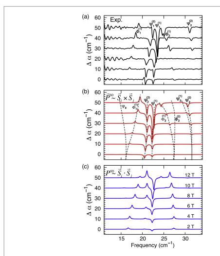
**Figure 3.** Origin of the strong NDD in BiFeO<sub>3</sub>. (a) The experimental NDD ( $\Delta \alpha$ ) with static magnetic field from 2 to 12 T and oscillating electric field along [1, -1, 0]. The predicted NDD using (b) SC and (c) ES polarizations. Here, i, j denote nearest neighbors.
