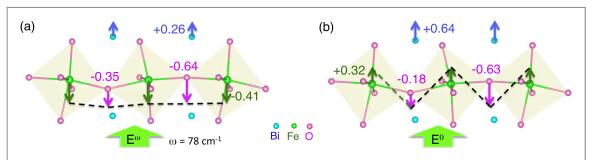
**Figure 4.** Distinct atomic responses to dynamic and static electric fields. The lowest-frequency eigenvectors of (a) dynamic and (b) force-constant matrices are compared. Note that the polar displacement in the dynamic limit ( $\omega = 78~{\rm cm}^{-1}$ ) increases the Fe–O–Fe bond angle (dotted line) while the displacement decreases the bond angle in the static limit.
