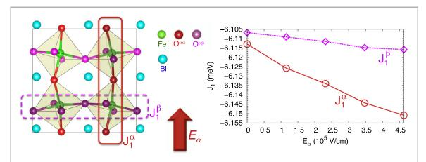
Figure 2. Strong anisotropic response of magnetic exchange  $(J_1)$  to an electric field. The slopes of thick and dotted lines represent derivatives of  $J_1$  with respect to electric fields parallel ( $C_{\parallel} = \partial J_1^{\alpha}/\partial E_{\alpha}$ ) and perpendicular ( $C_{\perp} = \partial J_1^{\beta}/\partial E_{\alpha}$ ,  $\alpha \neq \beta$ ) to the spin-bond direction calculated from DFT.
