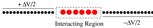
FIG. 1. (Color online) Schematic representation of the geometry used in our study. The leads are modeled by tight-binding Hamiltonians. The ground state at time zero is calculated at zero bias. Then, a finite bias \Delta V is applied between the two leads (without ramping time for simplicity, but this can be changed in future studies) and the resulting current is measured.
