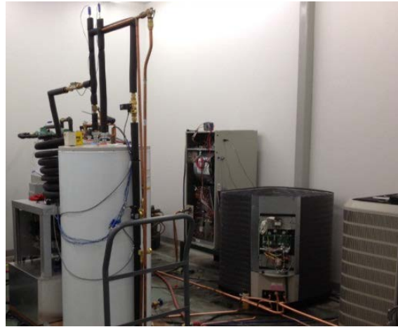
Figure 4. First Lab Prototype AS-IHP System; (l to r) Water Heating Section with Tank, Indoor Blower and Coil Section, Compressor Section, and Outdoor Fan and Coil Section
