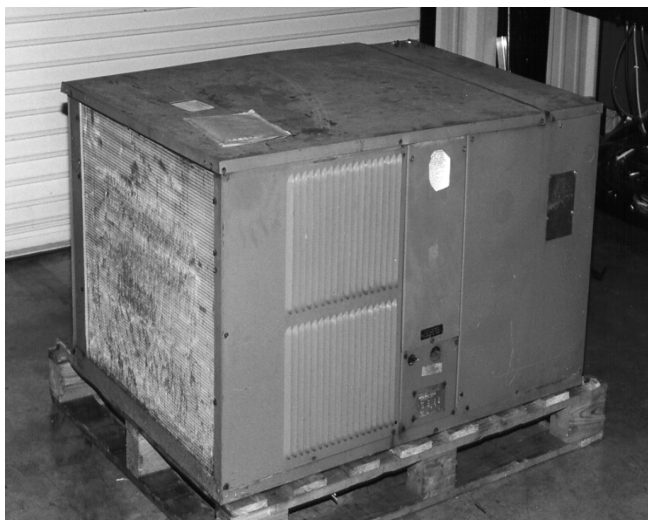
Figure 1 As-received single-package 15-year-old heat pump.
