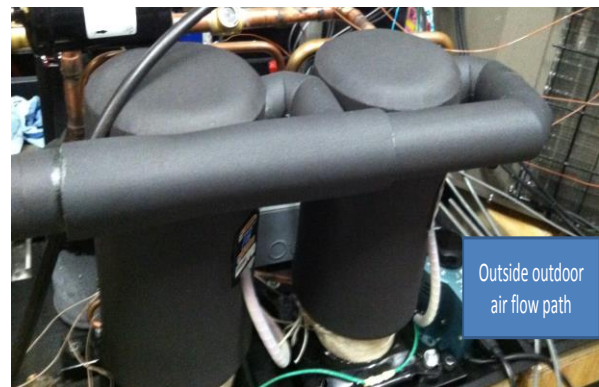
Figure 4 Left: CCHP using tandem, single-speed compressors and an EXV for discharge temperature control in heating mode, right: Insulated tandem, single-speed compressors
