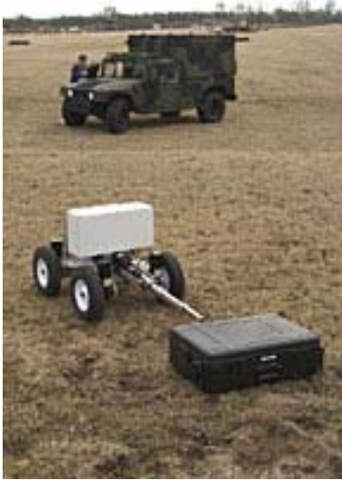
SRNL's MoPED is designed to disable or disarm Improvised Explosive Devices in Iraq and other military theaters.
