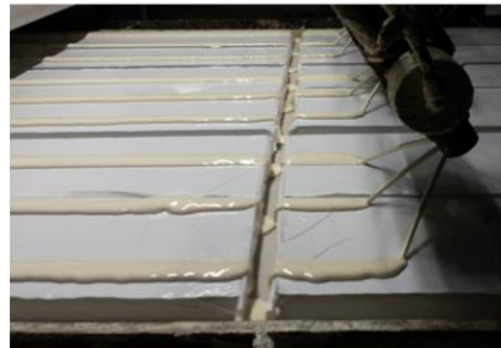
Foam application on manufacturing line
