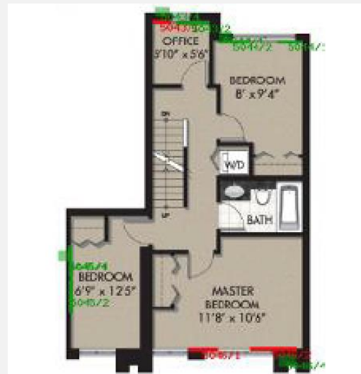
Figure 3: Sensors having elevated moisture content in the 2 nd floor of Townhouse 108.
