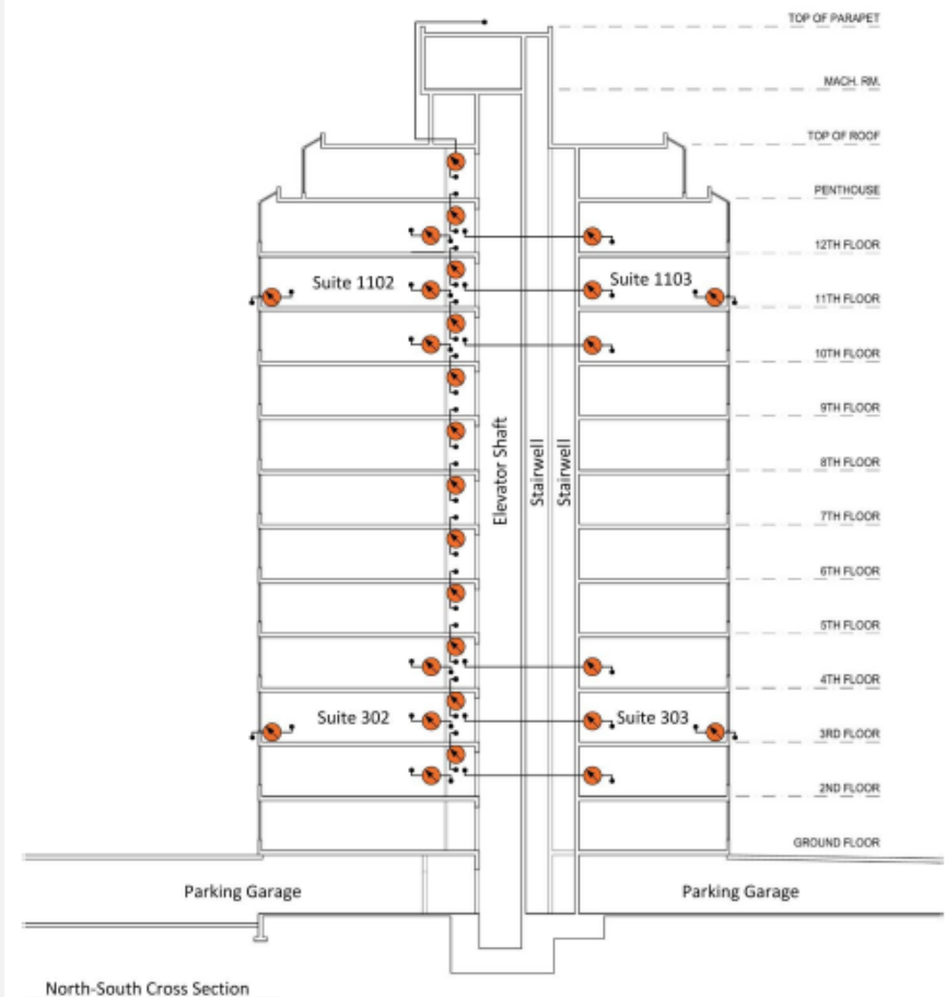
Figure 7-28: North-south cross-section of the case study building illustrating how the pressure measurements are linked
