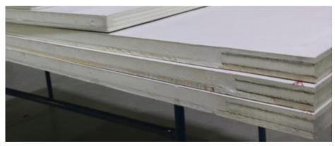
Finished composite insulation boards
