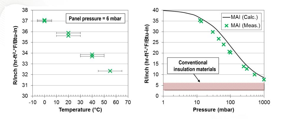
Even with complete loss of vacuum, MAI panels expected to have higher R/inch than conventional insulation materials.
