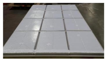
MAI panels attached to high-density (HD) foam substrate
