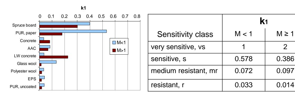
Very sensitive = pine sapwood (reference material) Experimental findings for growth intensity of different materials Scaling coefficients  $k_1$  for material sensitivity classes
