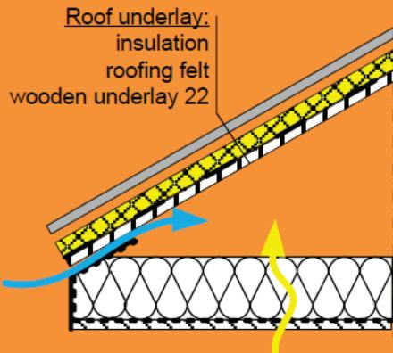
Insulated roof, some air leakage in the attic floor
