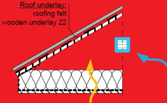
Reduced ventilation – only through gable vents; air tight roof eaves.
