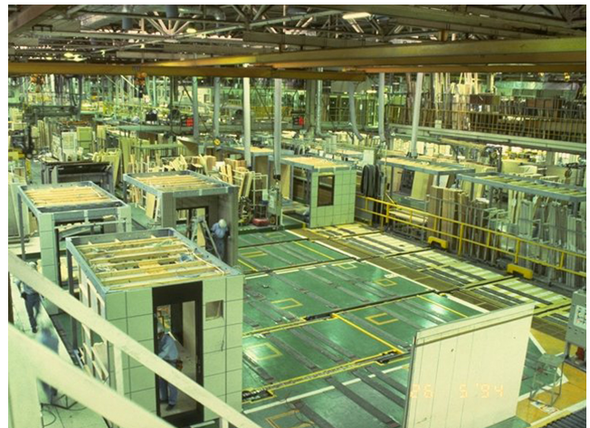
Figure 1 A volumetric production line.
