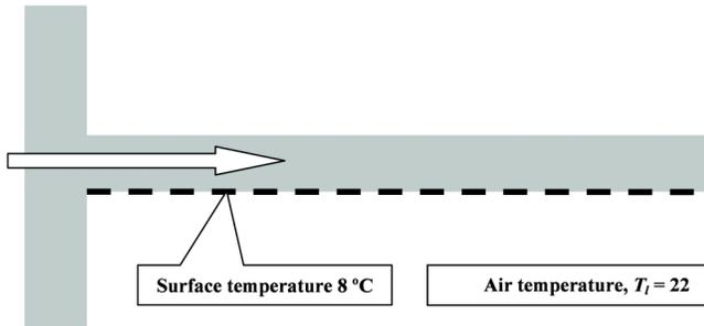
**Figure 3** Localized cooling of the ceiling as a result of air flow between the joists.
