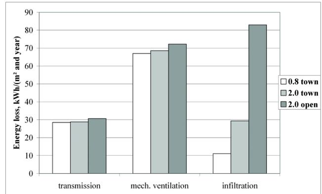
**Figure 2** Calculated energy losses for houses with airtightness according to the normal building code (in a town environment) and houses with a below standard airtightness according to the normal building regulations (town environment and open environment).
