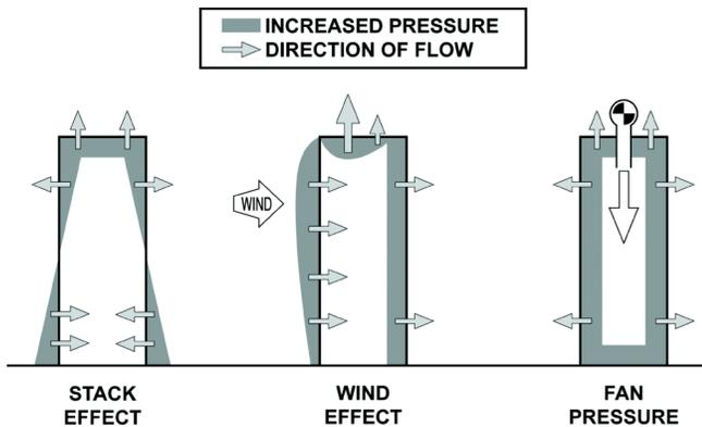
**Figure 1** Forces affecting air leakage.
