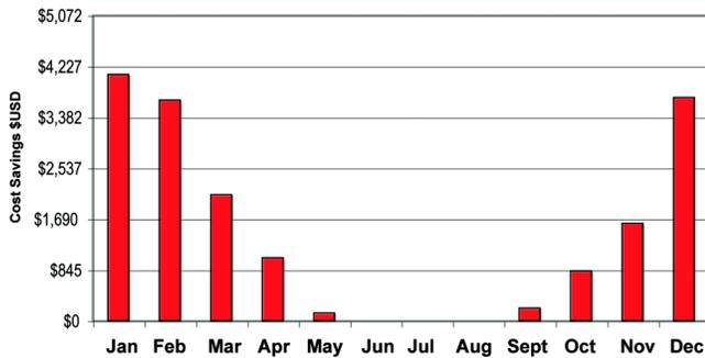
**Figure 2** Summary of energy-use calculation software analysis. This bar graph illustrates the forecasted cost reduction, by month, that will be attained by performing air leakage control retrofits to the building envelope.
