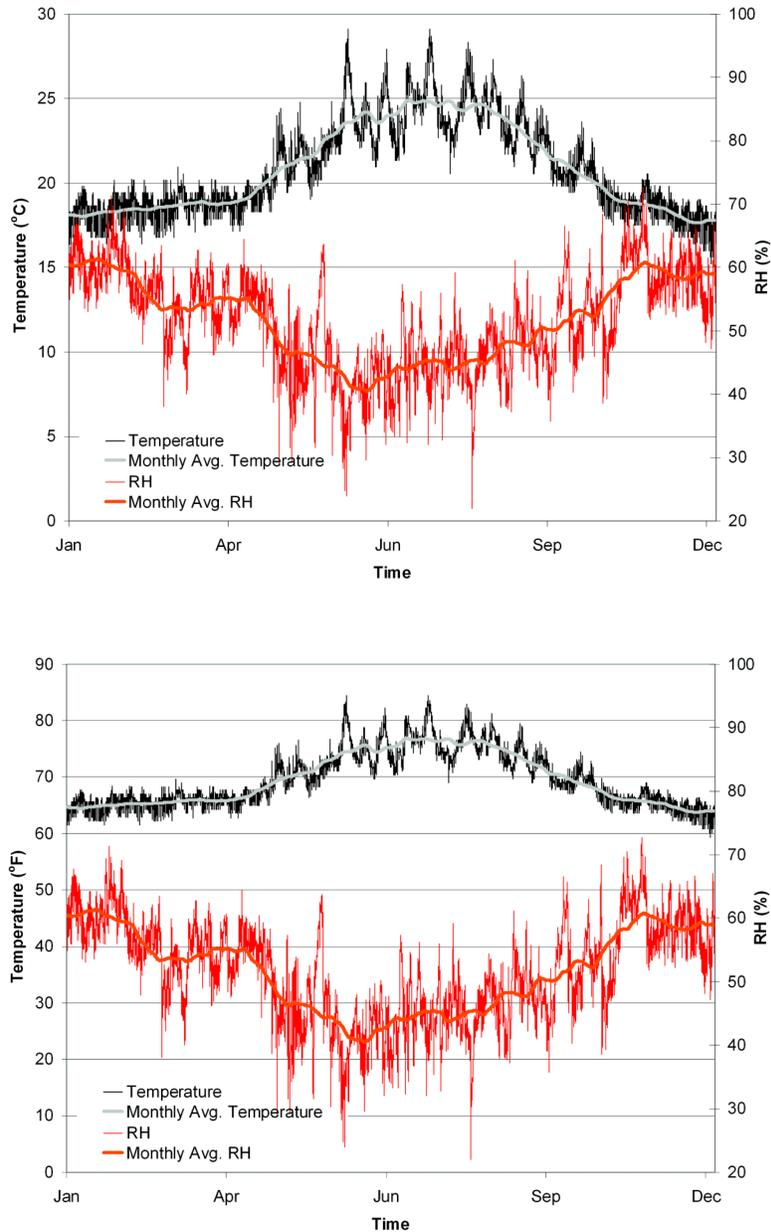
**Figure 3** Measured indoor conditions for a Vancouver multifamily building.
