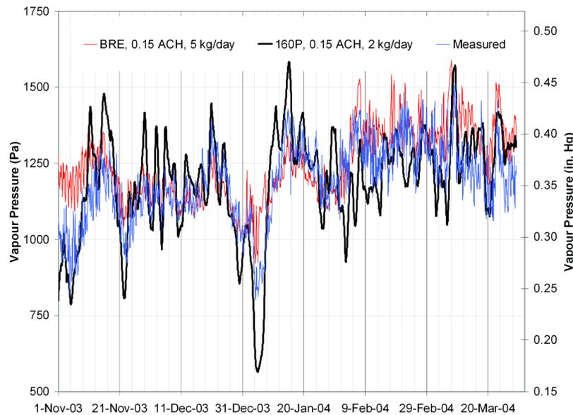
**Figure 1** Comparison of the 160P and BRE approaches to measured data of a multiunit residential building during the heating season for a mild marine climate (Vancouver).
