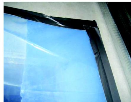
Figure 6 (a) The fan and pressure gauge fitted in a door opening to a stairwell and (b) sealing around a door.
