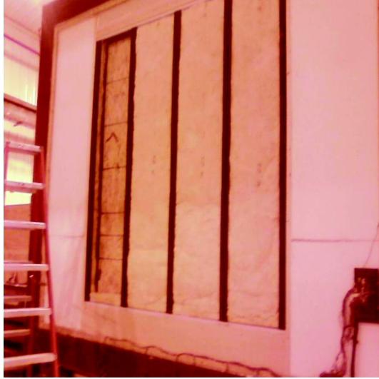
Figure 1 Configuration of the test steel stud wall using foam profiles and R-19 fiberglass batts.
