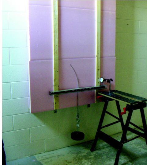
Figure 4 Laboratory mock up testing of deflection with load; 2 in. (51 mm) XPS foam and 1 × 3 strapping, 24 in. (610 mm) o.c.
