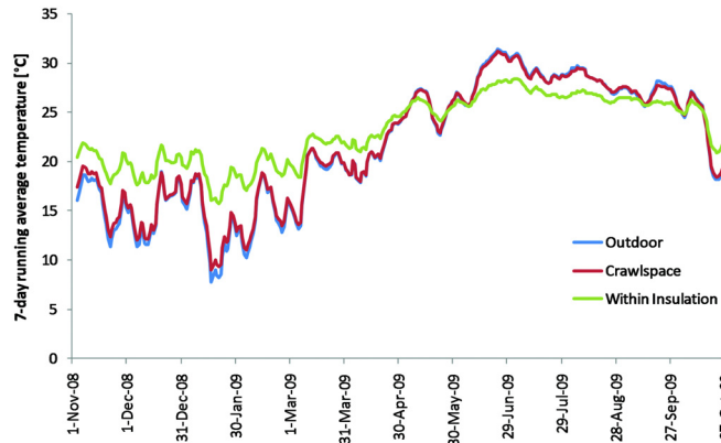
Figure 8 Seven-day running average temperature from data loggers placed outdoors, in the crawlspace, and within glass fiber batt insulation (House 1).
