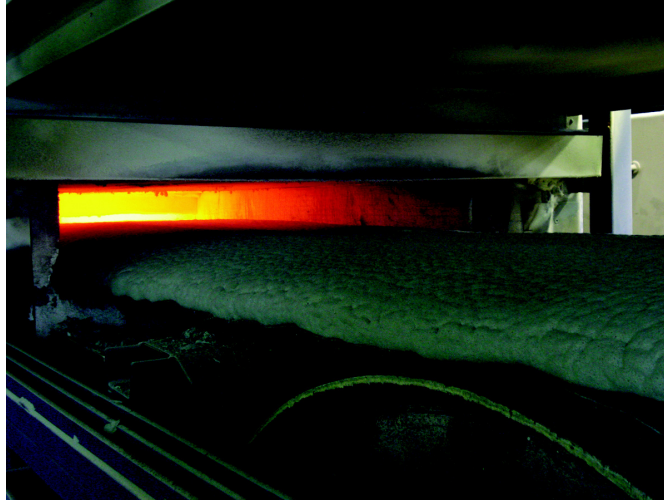
Figure 1 Exit point of the glass foam “cake” from the furnace. The expanded compound cools down from about 900°C to ambient temperatures. (Reproduced by permission of Misapor AG.)
