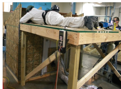
Figure 4 Mock attic structure with 5/12 gable roof, 4 \times 8 \times 4 ft chamber, door equipped with duct blaster, and working deck.
