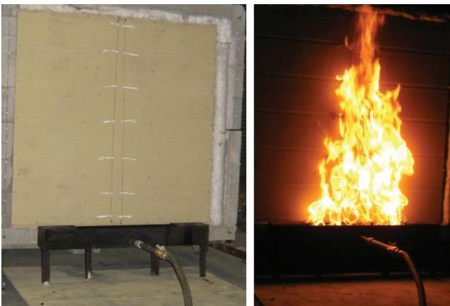
**Figure 8** Burner used for convective heating of the test samples.
