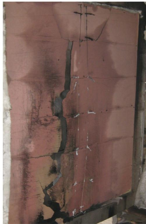
**Figure 18** Fiber cement board sample with XPS foam insulation at the end of the combined radiant and convective exposure test.
