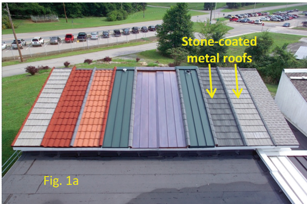
Figure 1 (a) Roofs offset-mounted from the roof deck for ASV or fastened directly to the roof deck on the Envelope Systems Research Apparatus. (b) Stone-coated metal offset from the roof deck using double battens.
