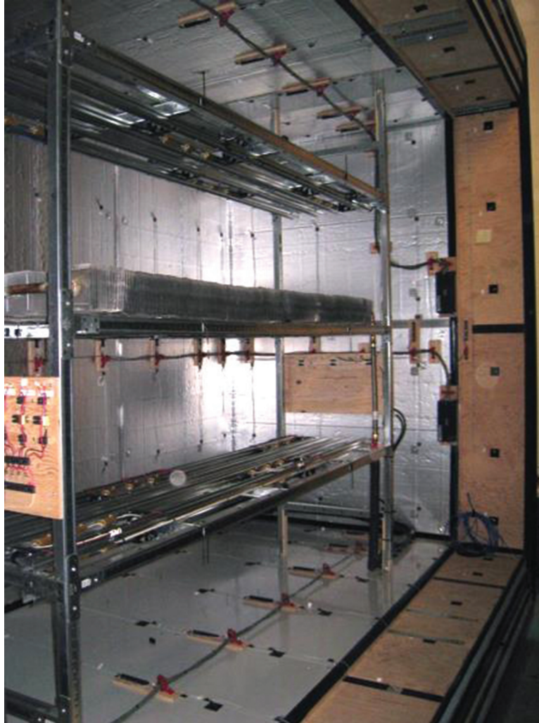
Figure 4 Upper and lower heating arrays and cooling coil mounted on a movable rack in the meter box.
