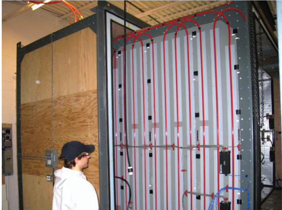
Figure 5 View illustrating the double-guarded concept: a conventional guard box on the left and an active liquid guard installed on the meter box on the right.
