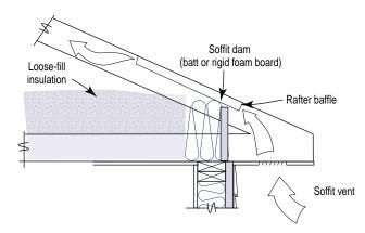
This oversized truss shows loose-fill insulation that is blocked or dammed at the eave with a soffit dam (a piece of fiberglass batt or rigid insulation). A rafter baffle creates a channel for air flow.
