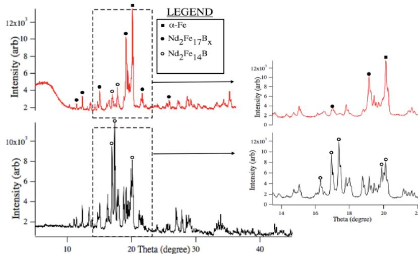
**Fig. 3.** XRD patterns obtained from the powder (shown below in black) and the build (shown above in red). Note the sharp decrease in the intensity of the peaks corresponding to the Nd<sub>2</sub>Fe<sub>14</sub>B hard magnetic phase in the additively manufactured samples. Also note the corresponding increase in the intensity in the alpha iron peak after laser processing [10].
