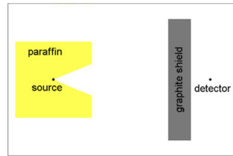
Fig. 16. Example of a two-material Ueki experiment, showing a cutaway view of the paraffin block.
