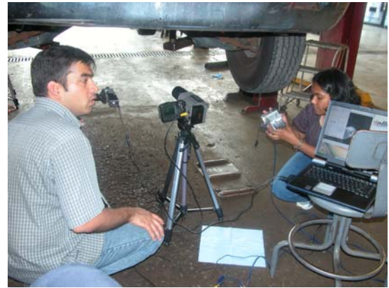
Figure 7. Setup for thermal data acquisition. The setup includes two uncooled infrared cameras, an infrared thermometer and a laptop for controlling the devices.
