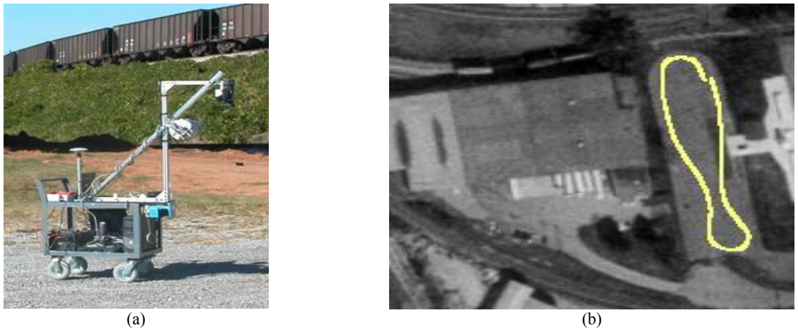
Figure 5: Real-time data collection. (a) Our multi-sensor integrated data collection system on a push cart. (b) GPS path (path length of 75 m) marked on a satellite image.
