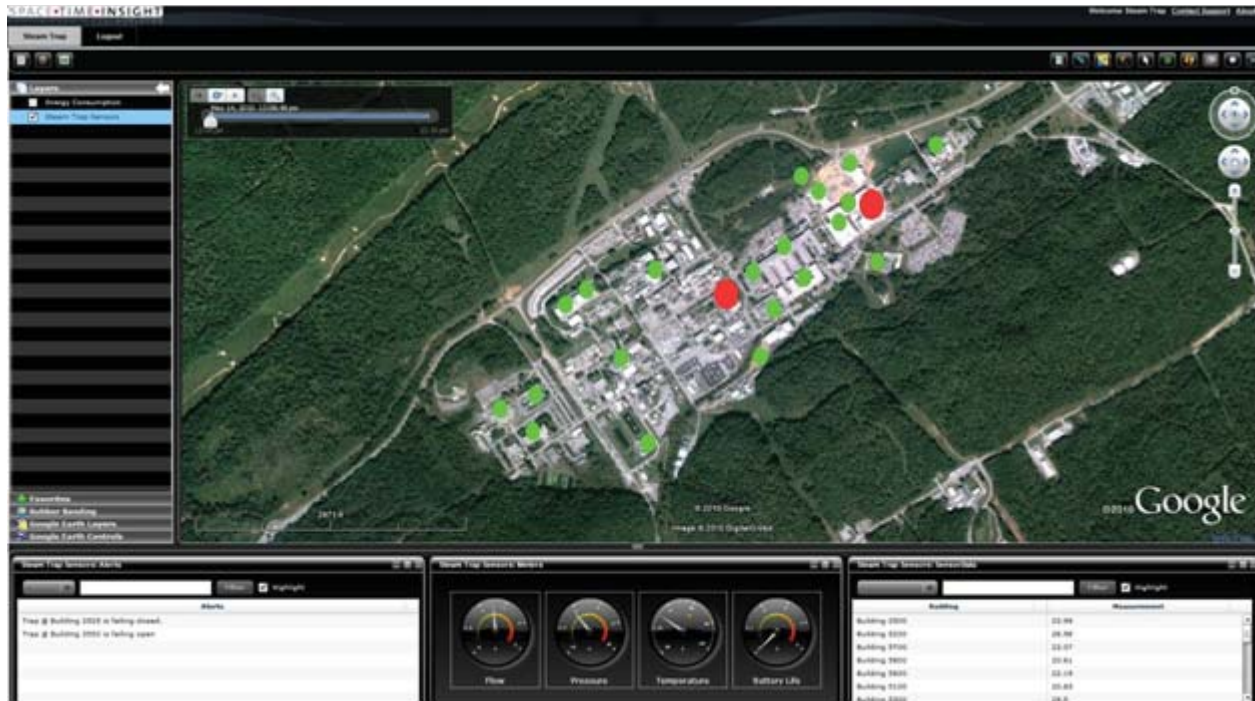
Figure 9. The situational awareness interface used to visualize sensor data from the wireless sensors along with status alerts.
